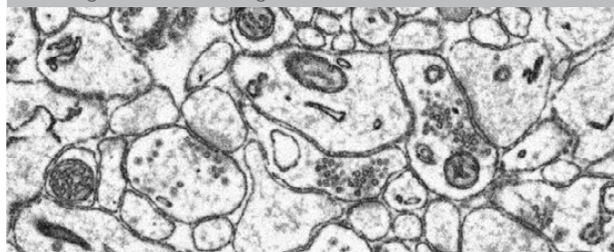
Mouse brain sample. Data acquired by physical slicing at HiVac mode. Imaged in BSE mode at 2 kV accelerating voltage, 0.1 nA beam current, 2 \mu s dwell time. Acquired pixel size 4 x 4 nm. Fine features as vesicles and synaptic clefts can be observed. With permission from Dr. Gabor Nyiri, Institute of Experimental Medicine, Budapest, Hungary.
