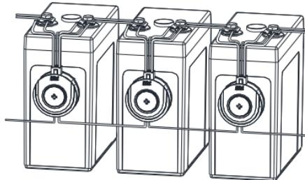
PBAT61 could be pasted on the battery surface, and connected with the battery poles by the standard 6pin cable securely, and cascaded with another sensor through RJ11.
