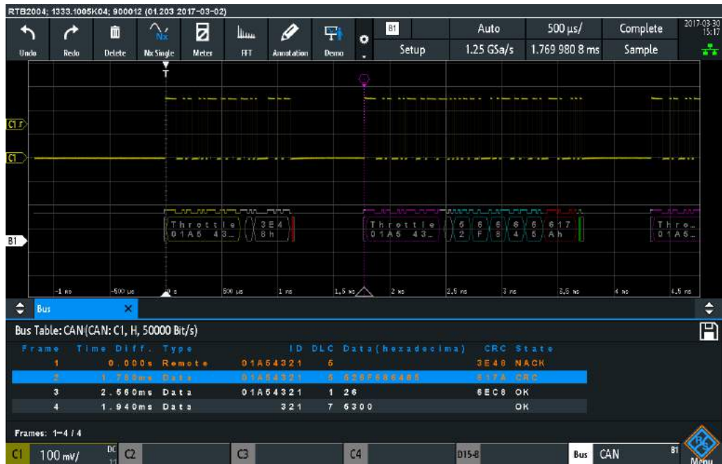
Figure 9-20: Decoded CAN signal with bus table and applied label list
