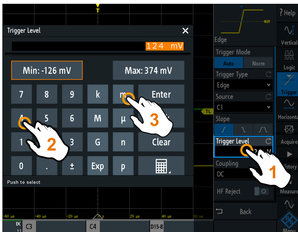
Figure 2-7: Enter numerical value and unit
