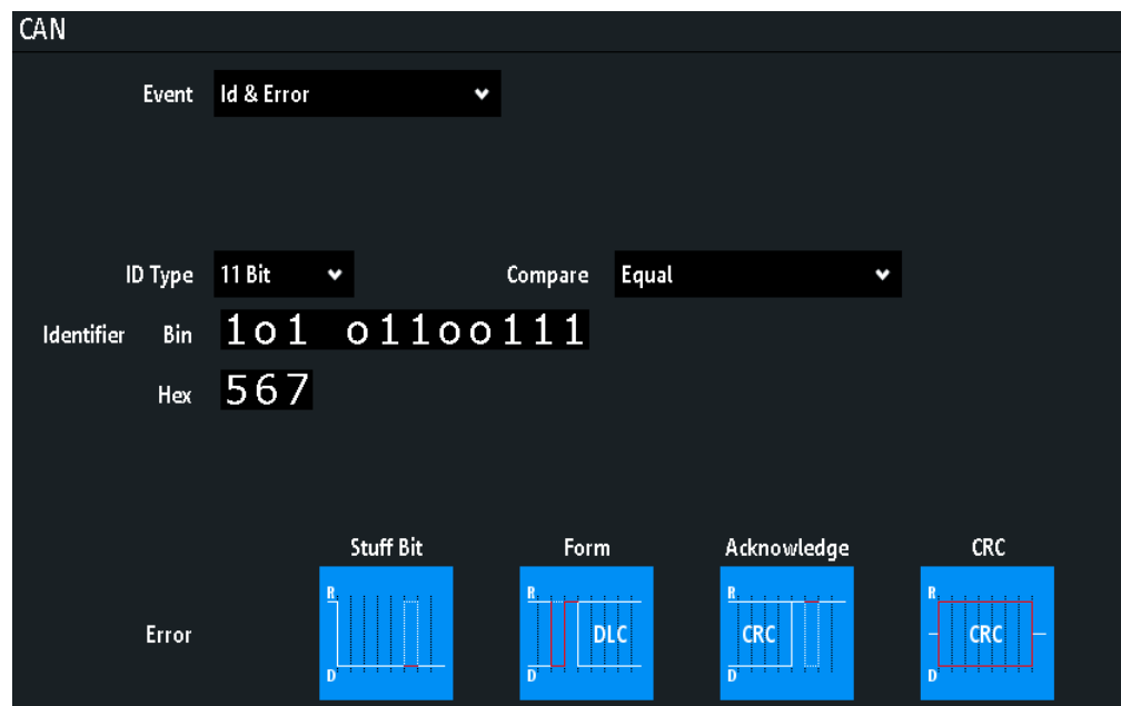
Figure 9-21: Search on CAN bus for frames with identifier 567 (hex) that have an error
