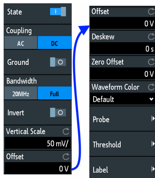
Figure 3-2: Vertical setup dialog, here split into two halves
