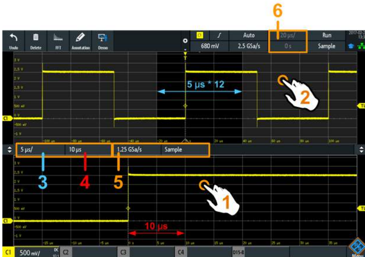
Figure 5-1: Zoom display: zoom is in the bottom window, normal waveform in the upper window
