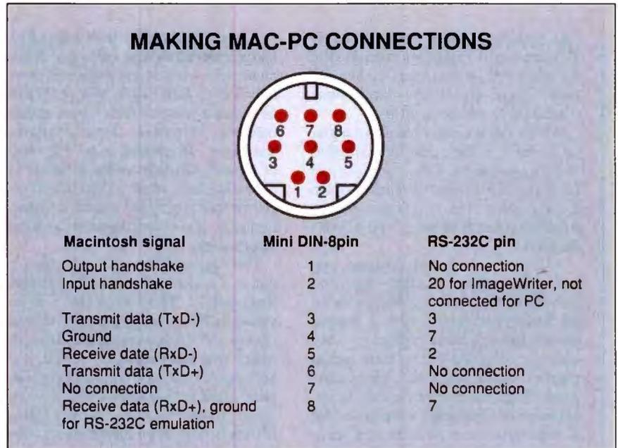
**Figure 1:** The schematic for a null modem cable to connect the serial ports of a Macintosh and an IBM PC. You can order an ImageWriter II extension cable and cut it in half to obtain the male DIN-8 connector. The DB-25 connector is available from most electronics stores.
