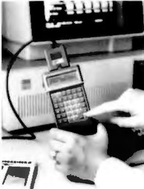
display, several different keyboard designs, and from 32K to 96K of internal RAM memory. All Organiser units can use our removable and interchangeable memory modules, allowing the Organiser II to be configured to meet your unique data and program memory requirements.
