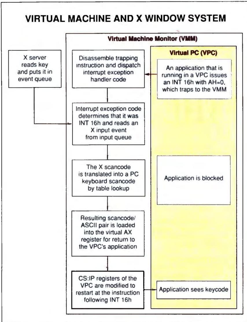
A virtual machine using an X window for its user environment. The X client is running separately on the host. The X server is wherever the user may be.
