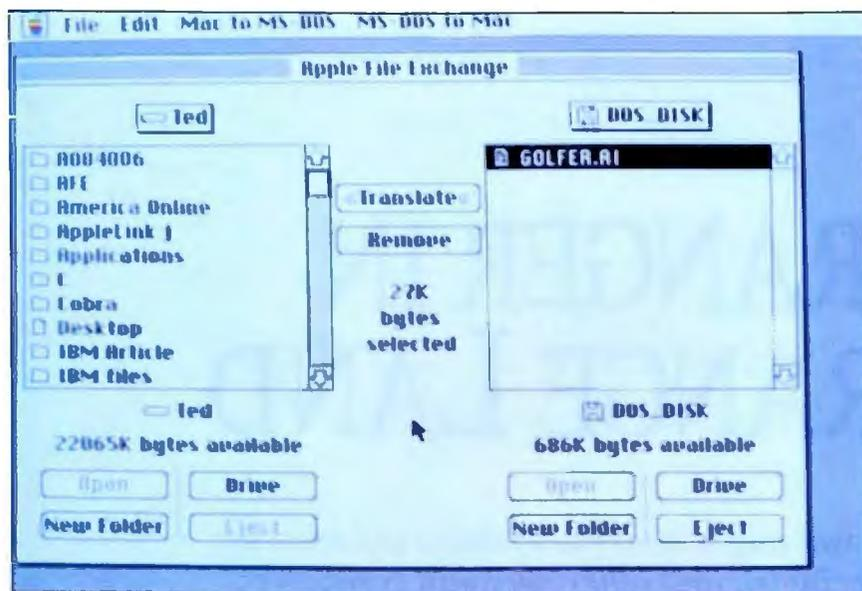
Photo 1: The Apple File Exchange program copying a file from an MS-DOS disk.
