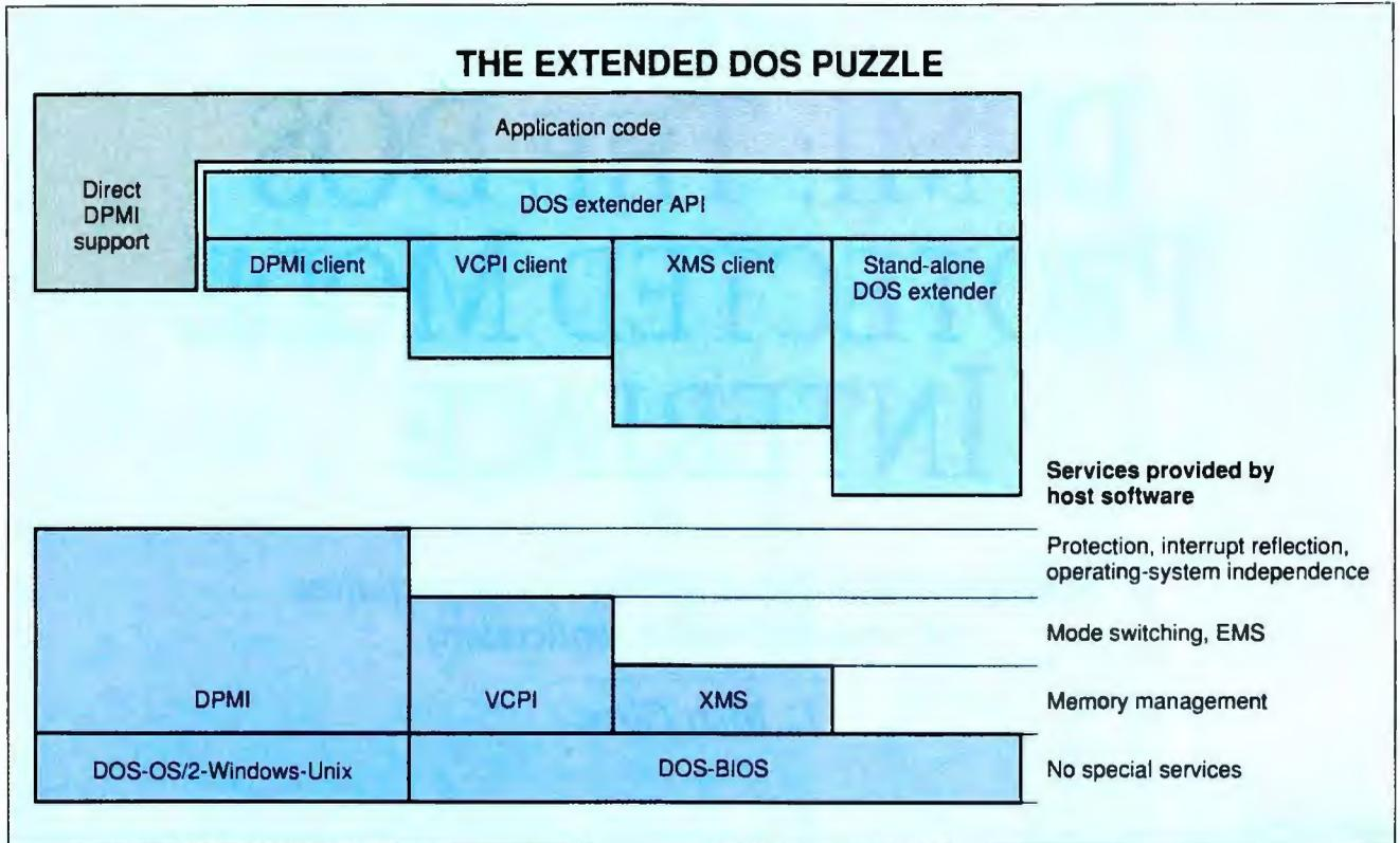
Many combinations and configurations of software run extended DOS applications. Here are all the services provided by the host environment, atop which runs the application.
