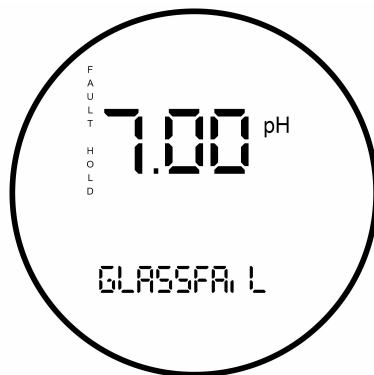
Figure 8-7: Disabling Fault Annunciation
