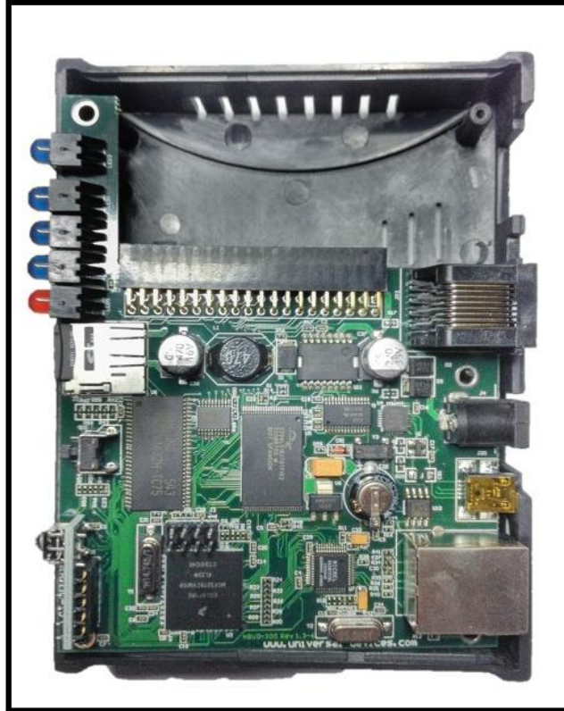
Figure 417: ISY with Cover Removed
