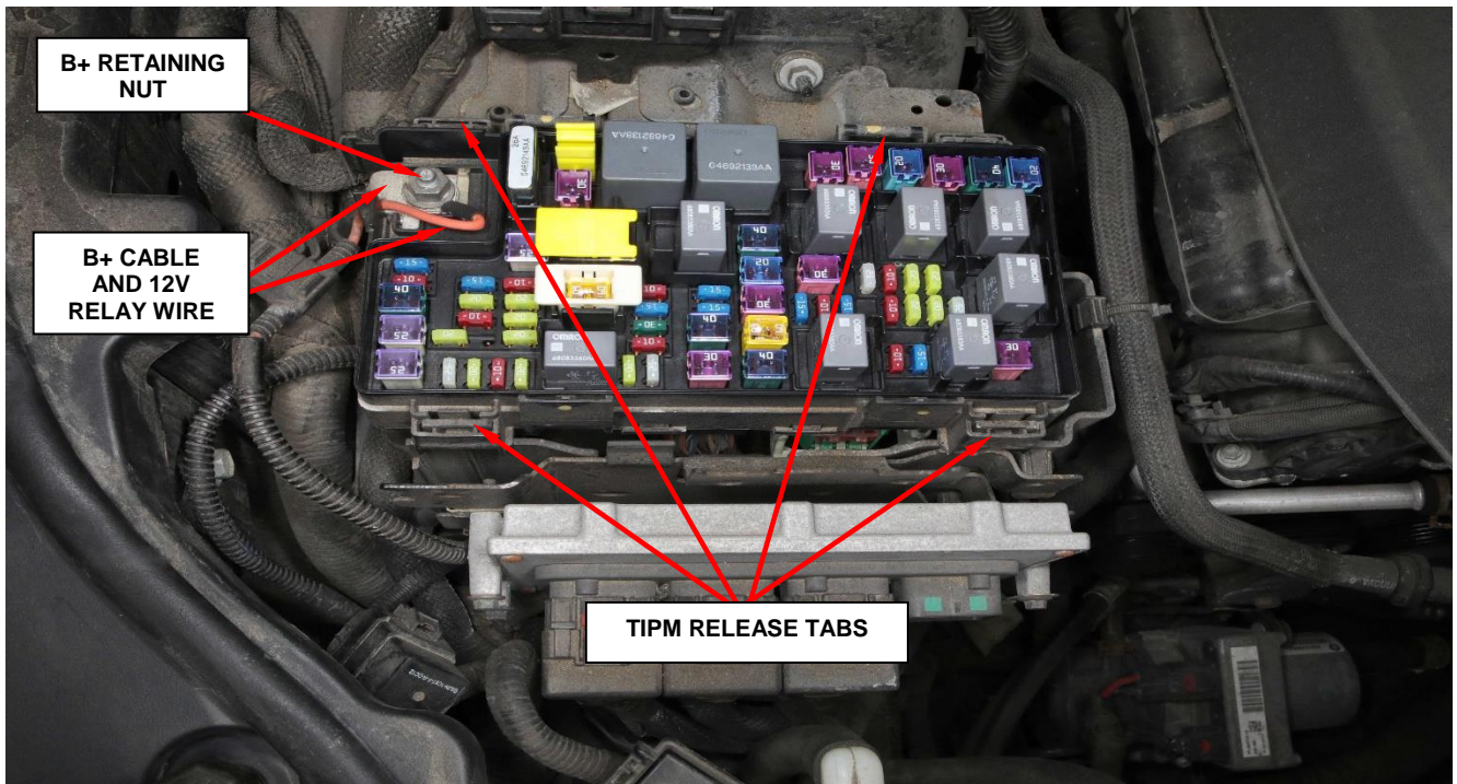
Figure 3 – TIPM Release Tabs
