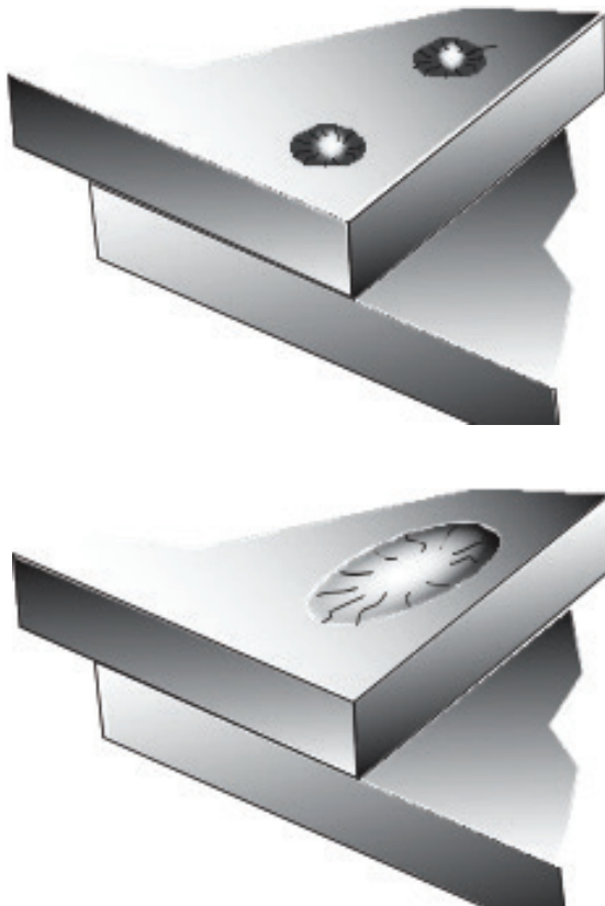
Plug Welds (Fig 1-19j)
