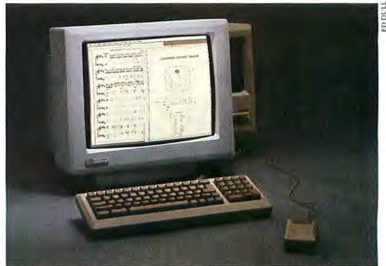
This 17-inch, 1024- by 808-pixel display from E-Machines lets you display more than one page at a time.
