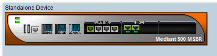
Figure 15-1: Mediant 500 MSBR Status Pane
