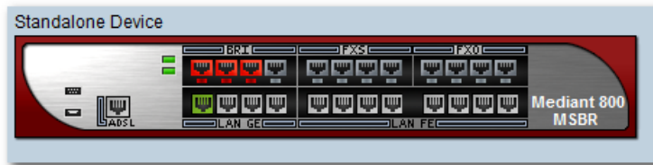
Figure 15-3: Mediant 800B MSBR Status Pane
