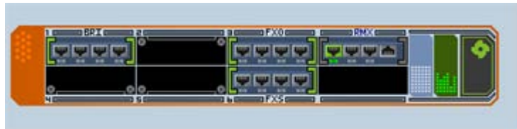
Figure 15-4: Mediant 1000B MSBR Status Pane
