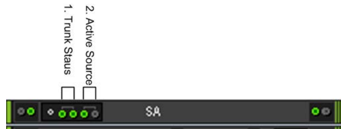
Figure 11-9: Mediant 3000 SA Board Status
