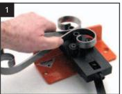
Riveting is simply achieved by placing the material to be joined (with rivet in pre-punched hole) between the riveting posts on the machine. Use the lever to squeeze up the rivet to form a strong joint.
