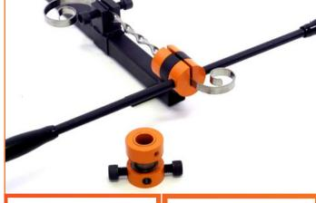
Use gripping bolts in collar and in the slide to set the section that you want to twist.
