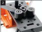
For the bending operation, material is placed between the square or diamond shaped former and the side rollers.
