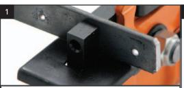
Punching is achieved by placing flat metal srip in the slotted punch block. Platform is adjustable to allow for accurate positioning along the center of different widths of metal.
