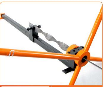
The Metalcraft XL Twister is available with an optional Basket Making attachment - allows one to produce top quality, robust baskets.
