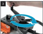
Rolling is achieved by using the winding handle to drive the bar forwards and backwards through the rollers. As this is done with each pass, the long lever is used to gradually increase pressure to roll an ever tighter curve. End stop screw and nut fitted for producing consistent bends and circles/arcs when rolling.
