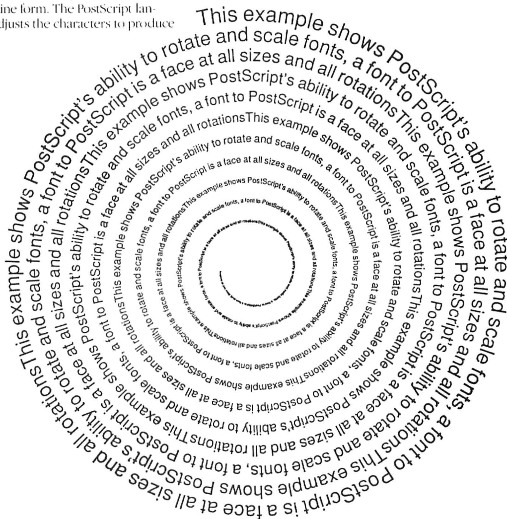
Infinity Circle This spiral of Helvetica characters was created on a VAX minicomputer and downloaded to a LaserWriter printer. You can't produce this design with MacDraw or MacPaint, but it illustrates PostScript's ability to produce fonts in any size or rotation.
