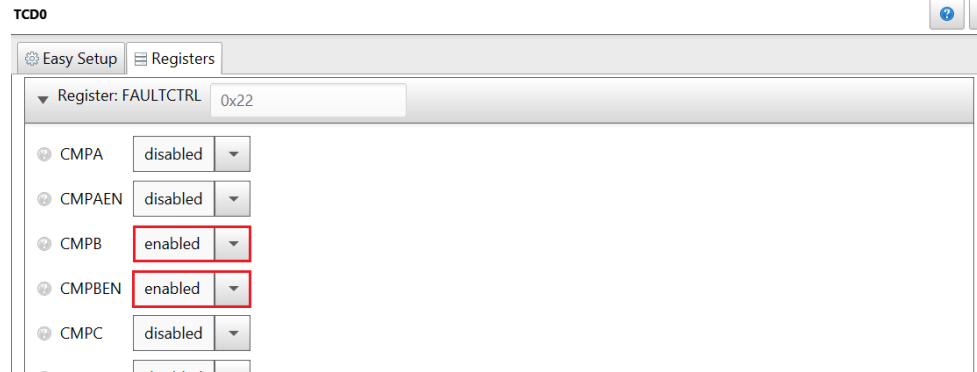
Figure 2-18. TDC0-Registers-CMPB and CMPBEN
