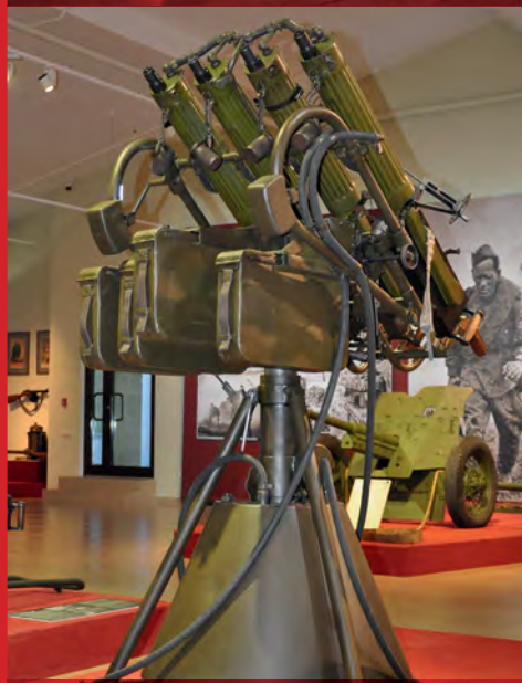
The '4M' quadruple 7.62mm 'Maxim' water-cooled anti-aircraft machine gun system was generally mounted on GAZ-AA and GAZ-AAA trucks for air defence purposes. This is believed to be the most complete surviving original 4M system
