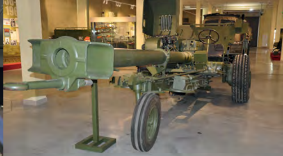
The 125mm 2A45 'sprut' was developed as an auxiliary propelled anti-tank weapon for VDV airborne forces, following the design principles of the similar 85mm SD-44 dating from the 1950s
