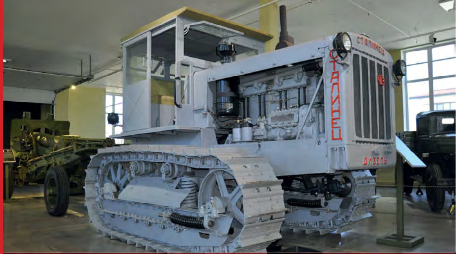
An S-65 artillery tractor. This particular vehicle was used after World War Two as an airfield tractor, and is fitted with the 'de-luxe' wooden cab. Few wartime S-65 driver-mechanics had the luxury of protection from the elements
