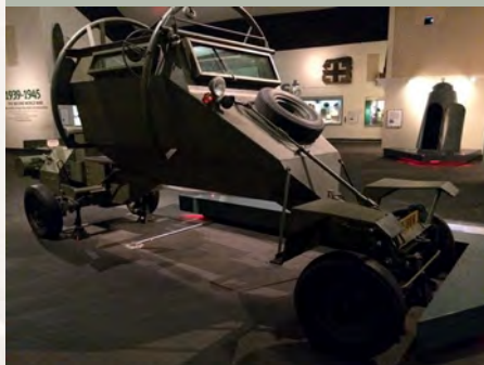
A 1979 Leopard Patrol Car, designed to keep its occupants safe from land mines. It had a V-shaped 8mm steel armour to deflect blast and 52mm bullet-proof glass
