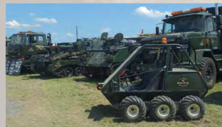
1986 RAF 'Vee-Pee' 6x6, built by French manufacturers Poncin to traverse marshland; part of the Walter Family collection, lined up behind
