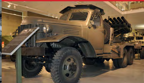
The BM-14 multiple rocket system (MRS), mounted on the ZIS-151 chassis, was a standard Soviet Army MRS in the 1950s
