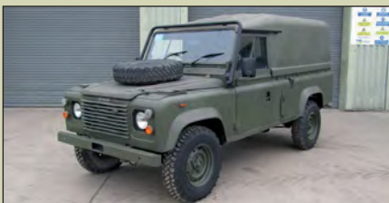
Land Rover Defender 110 Tithonus Hard Top RHD , Fitted 2500cc NAD engine LT77 5speed gear box, Transfer box with Hi Lo ratio & centre diff lock, 12 Volt electrics, Wolf style wheels, Disc brakes, Soft type steering wheel, mileage from 60,000 km, ..... Guide price from £8,250 (10 Available)
