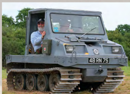
The Bombardier BR-100+ was designed specifically for use in snow, swamplands and desert terrains
