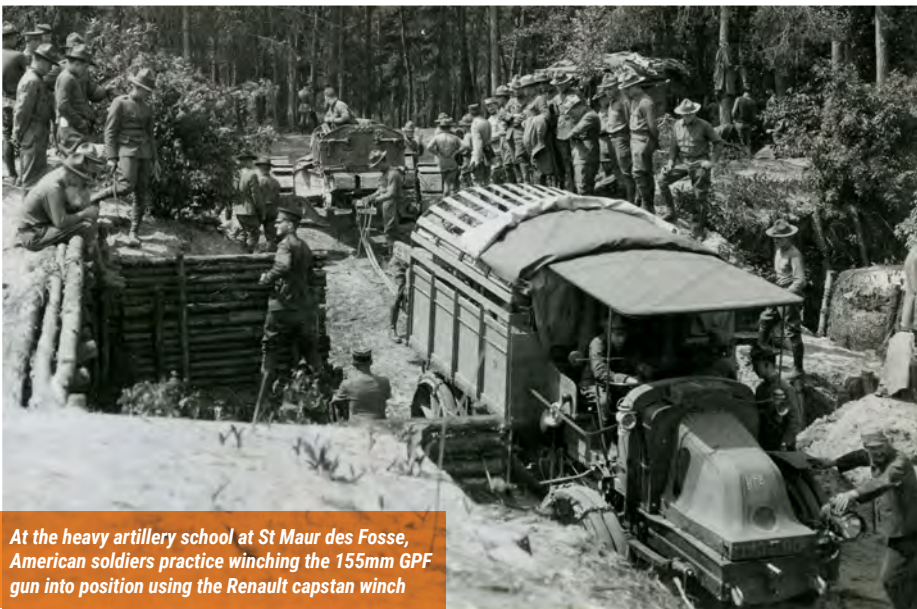
Weighing 13 tons the 155mm GPF gun was a heavy load. As can be seen here it had a handbrake and brakeman to help when going downhill
