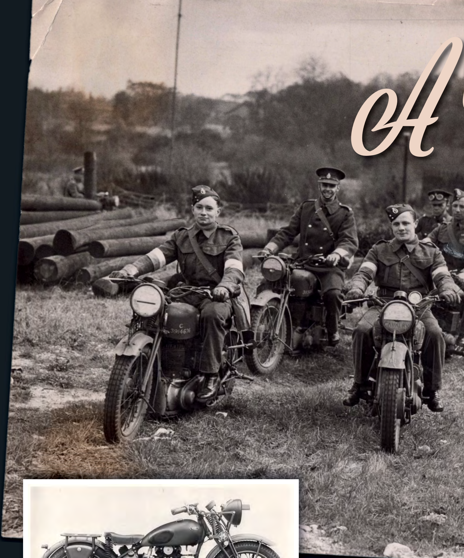
MAIN IMAGE: 1940: This photo issued on April 25, shows a group of Royal Army Signals Corps riders on a training exercise. They are riding BSA WD M20 motorcycles, a side valve single of 496cc displacement
