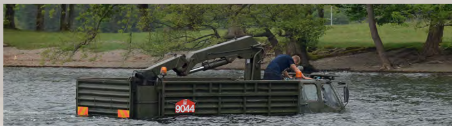
1972 Alvis Stalwart swimming. It has a Hiab crane, Rolls-Royce B81 engine and weighs nine tonnes
