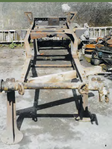
ABOVE: The sub-frame gets fitted to the main chassis, there are lots of subtle differences between the MKs
