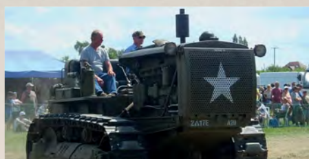
Armoured Caterpillar D2; these vehicles were produced from 1938-57 and had a four-cylinder Caterpillar diesel engine. Prestone 44 denotes the brand of antifreeze used and year it was put into the vehicle
