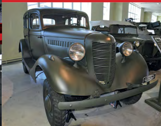
The 4x4 GAZ-61-73 all-terrain transport vehicle was built in small numbers at GAZ, but production was cancelled in the autumn of 1941 in favour of more urgent T-60 light tank assembly
