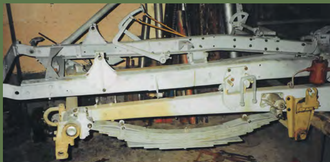
ABOVE: The sub-frame gets fitted to the main chassis, there are lots of subtle differences between the MKs
