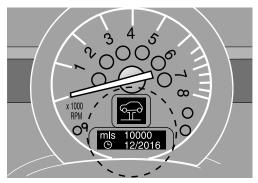
The remaining driving distance and the date of the next scheduled service are displayed briefly immediately after you start the engine or switch on the ignition.
