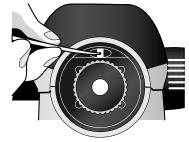
Unscrew the eyepiece cover  $\bf 5$ . Using the adjusting pin  $\bf 18$ , turn adjusting screw 5 clockwise or anticlockwise, until the calculated set value for height  $\bf b_2$  is reached when measuring on levelling rod  $\bf B$ .
