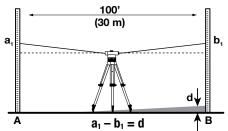
Set up the measuring tool in the centre and levelling rods A and B at both ends of the measuring distance.
