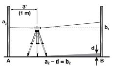
Set up the measuring tool approx. 6 ft (2 m) away from levelling rod  $\bf A$ . After aligning and focussing the measuring tool, read the height  $\bf a_2$  at levelling rod  $\bf A$ .
