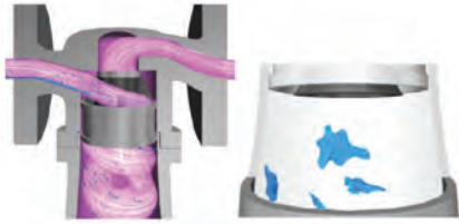
FIGURE 6. High-velocity cyclone separators can remove 98% wetness from steam provided that the flow velocity and wetness percentage are within the separator's required operating specifications
