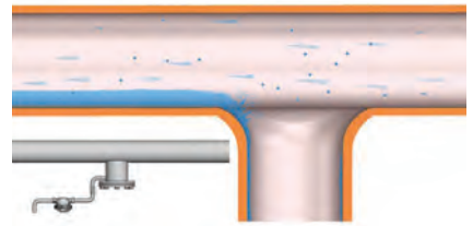
FIGURE 3. Steam contains condensate, both entrained in vapor, and disentrained flowing along the bottom of the pipe as a liquid stream. Only already disentrained condensate is removed through condensate discharge locations
