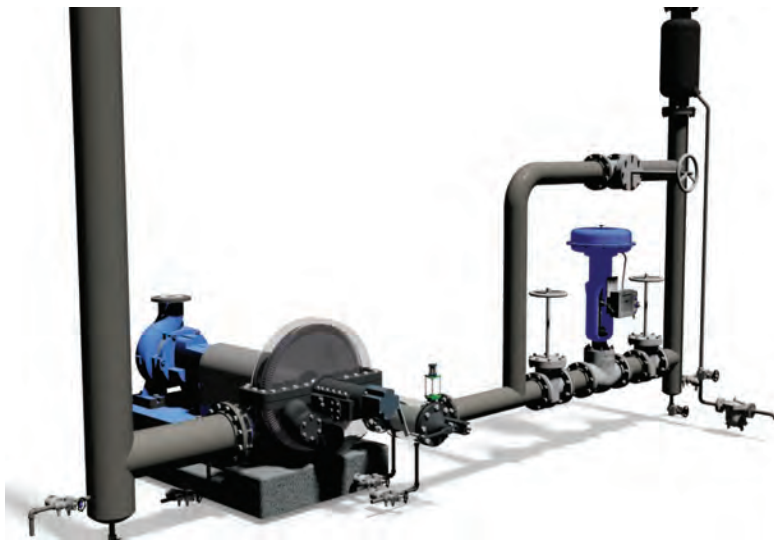
FIGURE 9. A turbine installation with properly drained and separated steam supply promotes reliable operation
