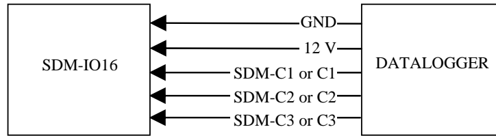
a) Connection with Datalogger Supply
