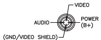
VIEW E-E SHOWN FROM PIN VIEW
