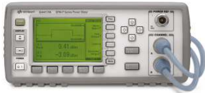
Figure 14. E4417A power meter configured to show a trace display (upper window) and a dual numeric display (lower window).
