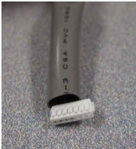
[CZ 7pin (Female)] Connect to the Canon MFP device
