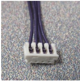
[CT 4pin (Female)] Connect to the Canon MFP device
