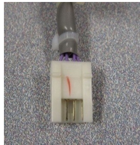
[EI 4pin (Male)] Connect to the 3 rd party external device
