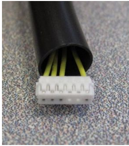
[CT 6pin (Female)] Connect to the Canon MFP device
