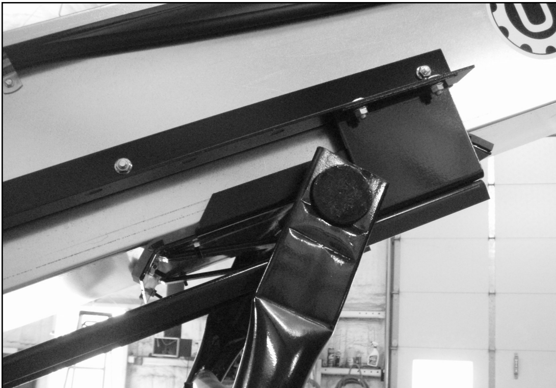
Picture of Slide Assembly after Installation
