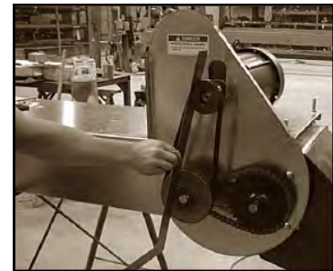
Lay a straightedge across pulley faces
