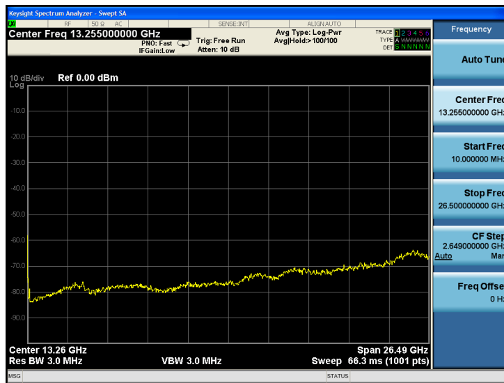
Figure 7-10. Rise in noise floor indicates changes in sensitivity with changes in LO harmonic used
