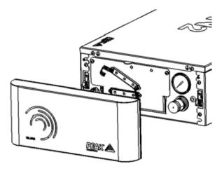
To access the regulator, unclip the fascia from the unit.
