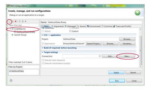
4. Upon selecting **New**, a **Select Remote System Type** window appears. In the **Select Remote System Type** window, expand **CodeWarrior Bareboard Debugging**, then select **Hardware or Simulator Connection**, and then click **Next**.
