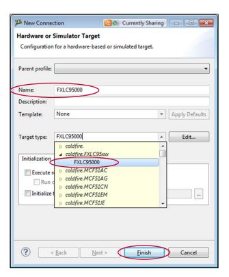
7. In the **Hardware or Simulator Connection** window, from the choices available in the **Connection type** menu, select the **P&E ColdFire multilink** (exact wording may be different), and then click **Finish**.
