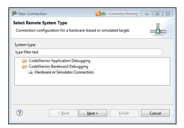
5. In the **Hardware or Simulator Connection** window, enter **FXLC95000\_multilink** into the **Name** field, and then click **New**, located to the right of the **Target** field.
