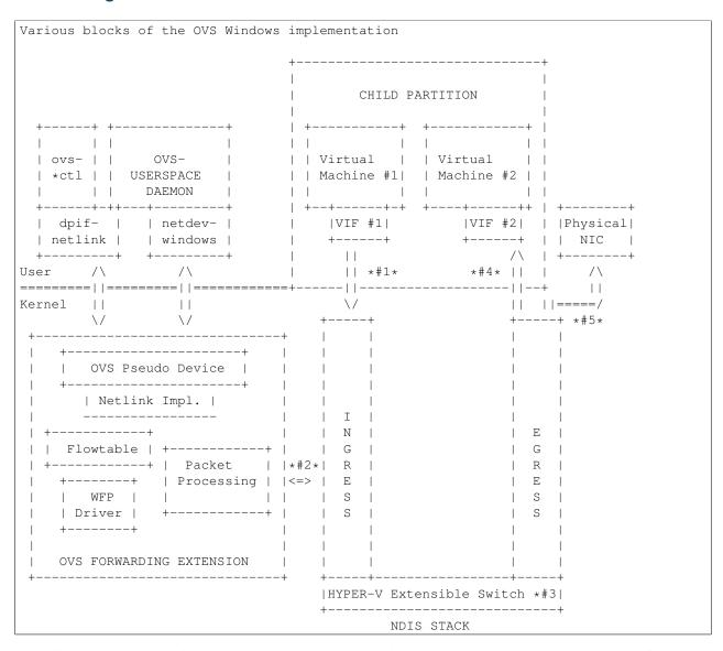
This diagram shows the various blocks involved in the OVS Windows implementation, along with some of the components available in the NDIS stack, and also the virtual machines. The workflow of a packet being transmitted from a VIF out and into another VIF and to a physical NIC is also shown. Later on in this section, we will discuss the flow of a packet at a high level.
