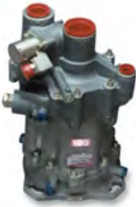
Engine Driven Pump
