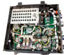
Power Distribution Unit
