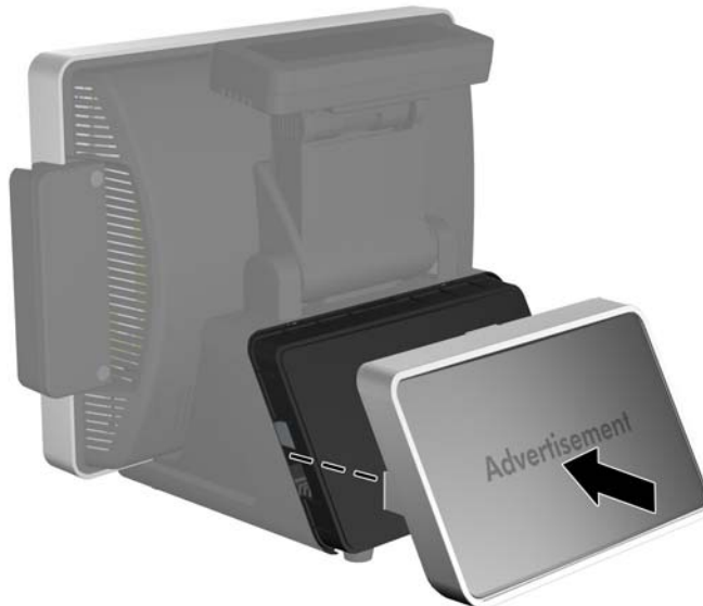
Figure 7-8 Replacing the Print Advertisement Panel Cover
