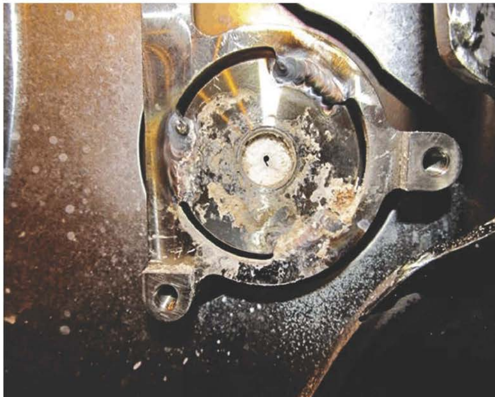
Figure 1. Normal DEF Crystallization in the DEF Doser Port Hole
