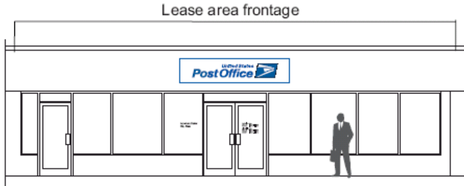
Exhibit 3-8a Elevation of sign placement for Alternate Quarters
