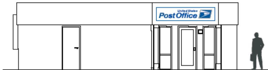
Exhibit 3-7c Typical elevation of Modular Building sign placement
