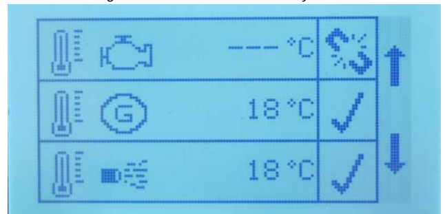
Fig. 11.2.1.1-1: Sensor defect symbolic
