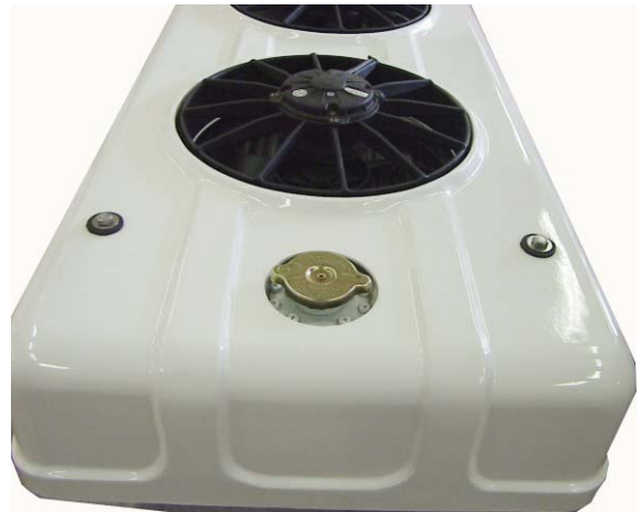
Fig. 7.6-4: Cooling water filler cap
