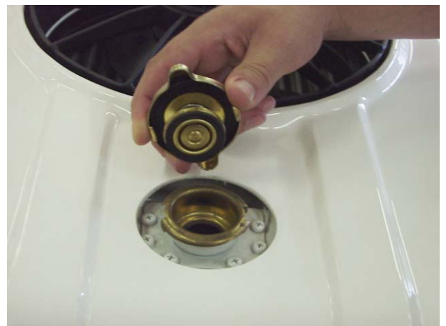
Fig. 7.6-5: Cooling water filler cap
