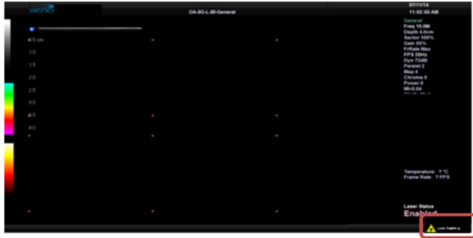
Figure 114: Laser State Message Shows Laser Emitting. Foot switch is pressed and the OA/US Probe is emitting laser energy.
