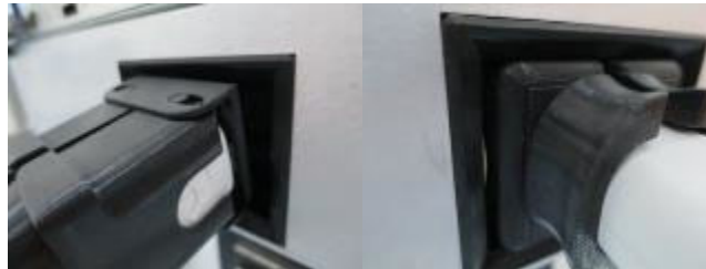
Figure 102: Inserting the OA/US Probe with Properly equipped OA/US Probe Calibration Adapter into the Calibration Port
