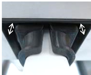
Figure 103: Properly Seated: OA/US Probe with equipped OA/US Probe Calibration Adapter flush with the Power Sensor Shield
