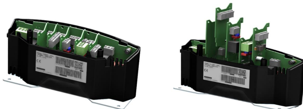
Figure 23: Inside view of the Next Gen CoreSense module, with the modular boards
