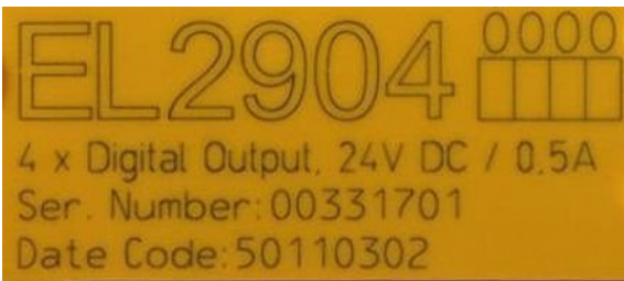
Fig. 34: EL2904 IP20 safety terminal with batch number/ date code 50110302 and unique serial number 00331701
