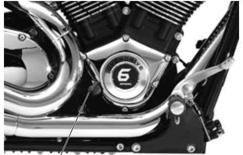
Oil Fill Cap/Dipstick
