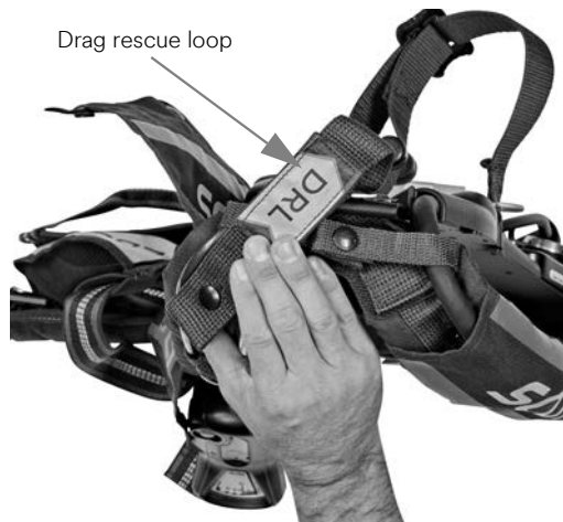
Figure 2-2 Unsnapping the drag rescue loop from the shoulder pad
