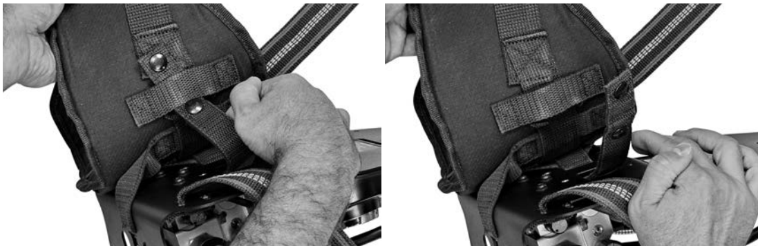
Figure 2-12 Sliding the waist pad retaining strap through the waist pad loop
