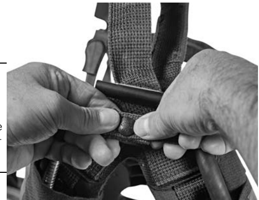
Figure 2-28 Securing the cables and hose
