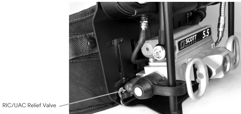
Figure 1-2 Inspecting the RIC/UAC connection
