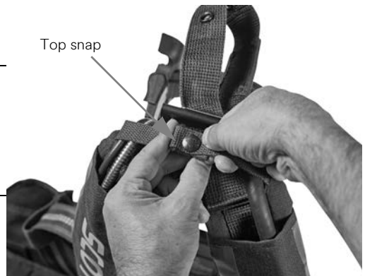
Figure 2-3 Unsnapping the top strap securing the cable, gaugeline, and regulator hose
