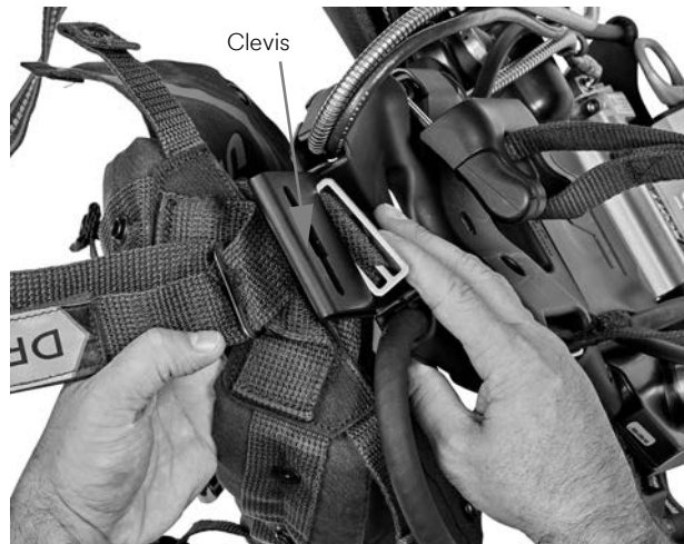
Figure 2-23 Passing the lower metal slide through the lower slot of the clevis
