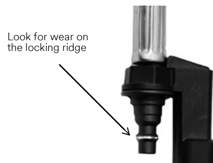
Figure 1-6 Inspecting the male quick-disconnect
