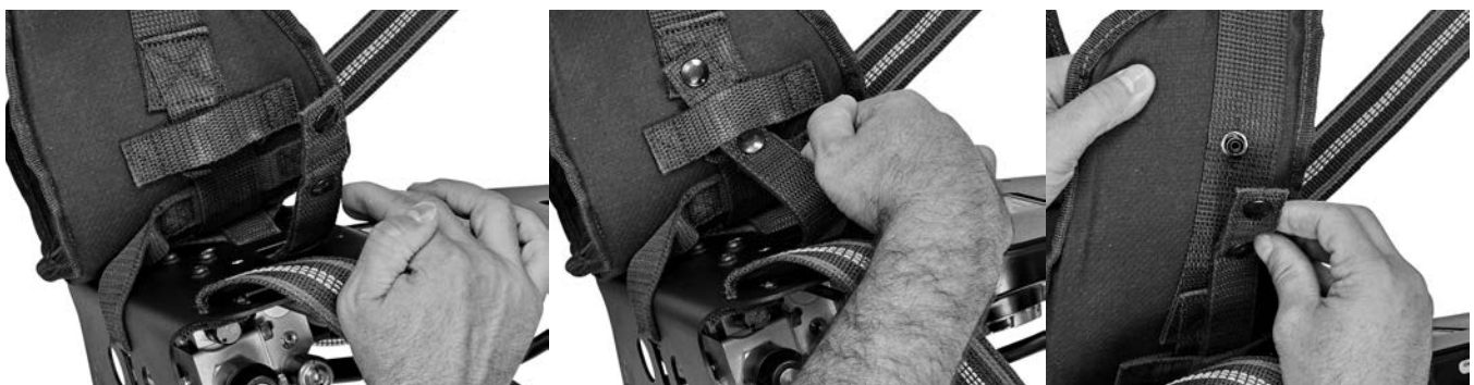
Figure 2-20 Threading the waist pad retaining strap through the waist pad loop and snapping it into place
