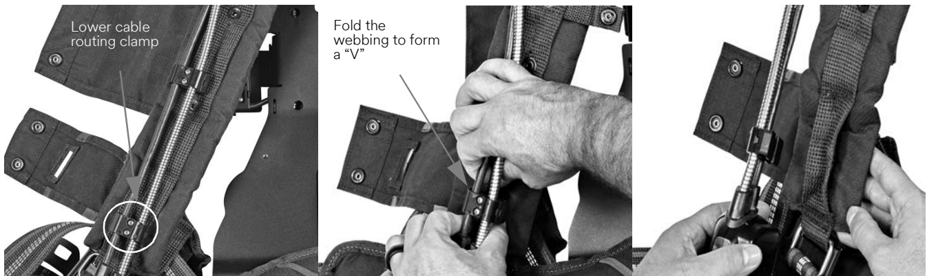
Figure 2-4 Removing the lower cable routing clamp
