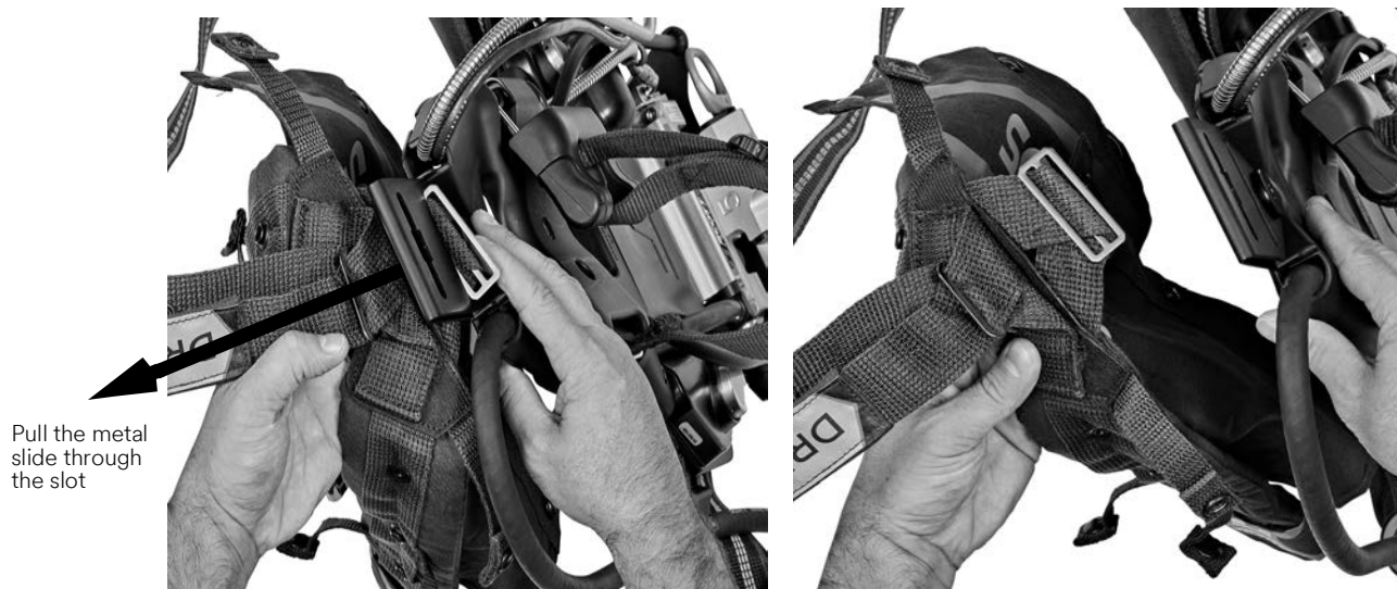
Figure 2-9 Pulling the lower metal slide through the lower slot of the clevis
