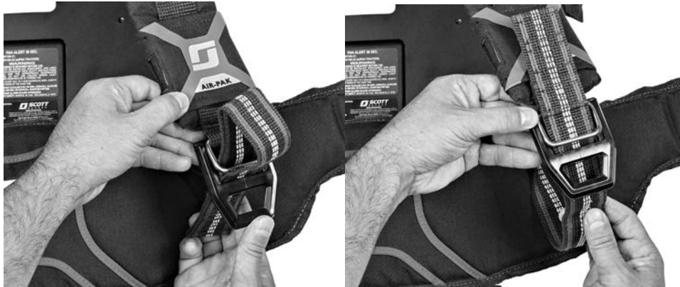
Figure 2-6 Detaching the waist-to-shoulder straps
