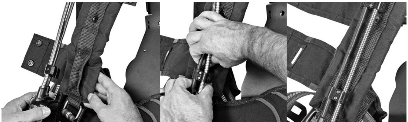
Figure 2-27 Attaching the lower cable routing clamp
