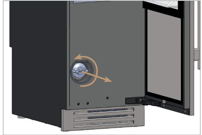
FIG. 1. Rotate the existing water filter counterclockwise.
