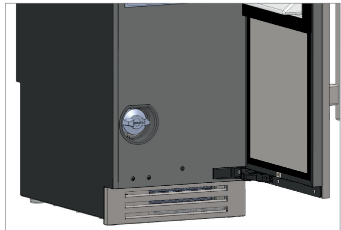
FIG. 3. Installed water filter.
