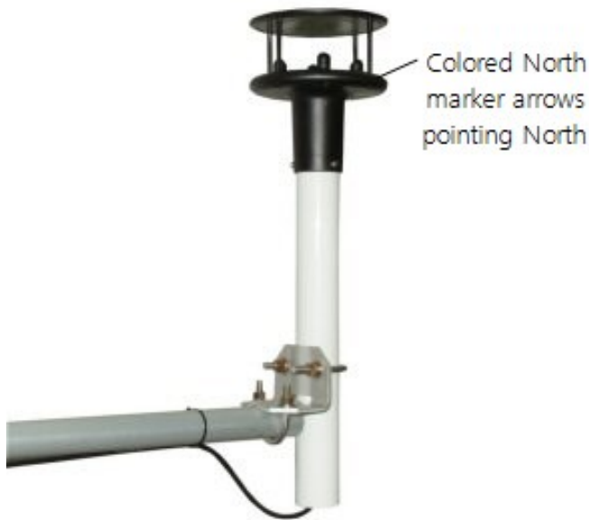
FIGURE 7-1. WindSonic4 mounted on a crossarm
