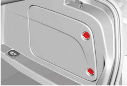
Battery Access Panel
