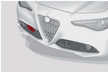
Front Bumper Radar Location
