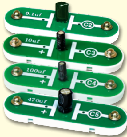
Capacitors (C2, C3, C4, & C5)
