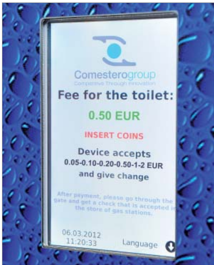
Colored LCD 7" monitor displays all necessary informations for the users
