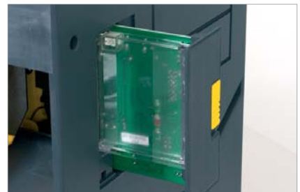
Board easily extractible from the outside
