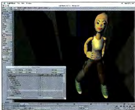
Skin and Bones Inverse and forward kinematics, and a new motion mixer, can be used to control a character's skeleton.
