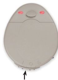
Fig. 4 The RONDO in ON position
