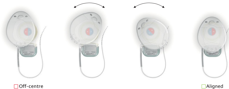
Fig. 11 Aligning audio processor and implant magnets. Note that the microphone is facing up.
