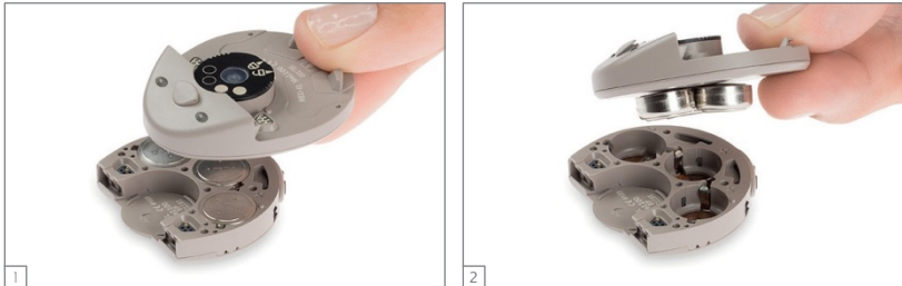
Fig. 16 Changing the batteries of your audio processor
