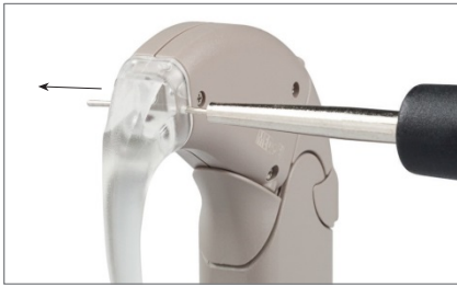
Fig. 21 How to remove the earhook pin
