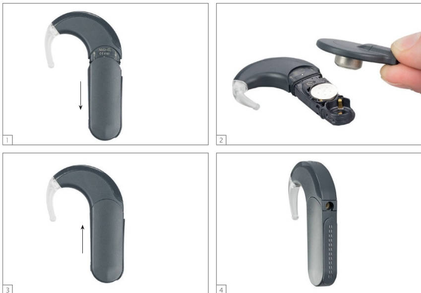
Fig. 35 Changing the batteries of your audio processor
