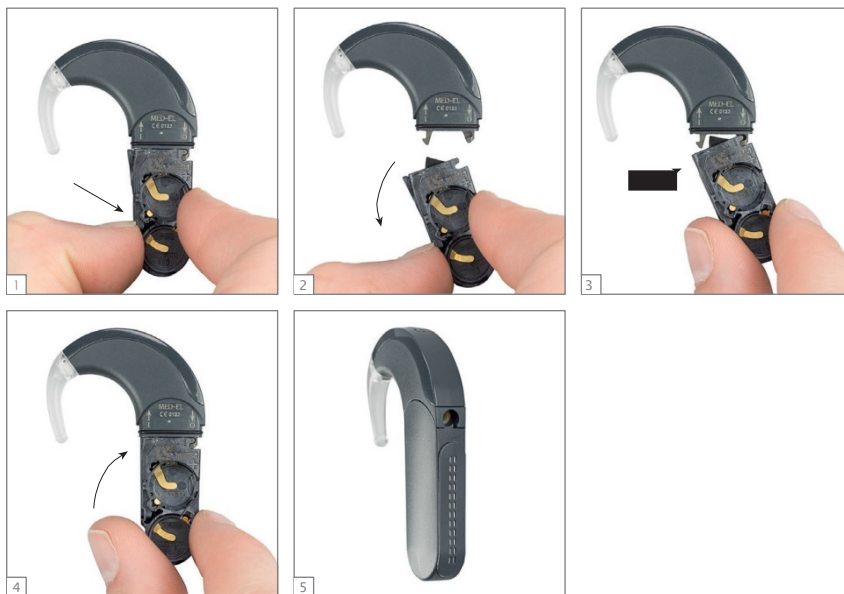
Fig. 10 How to remove/attach the battery pack from/to the control unit
