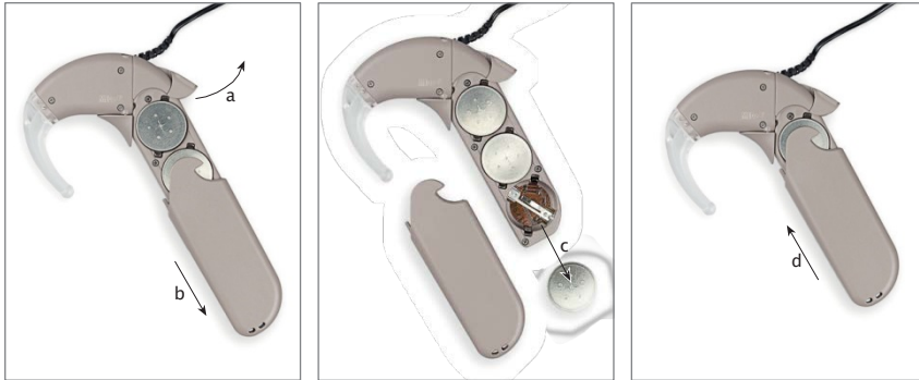
Fig. 24 Changing the batteries of your audio processor
