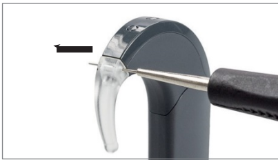
Fig. 31 How to remove the earhook pin
