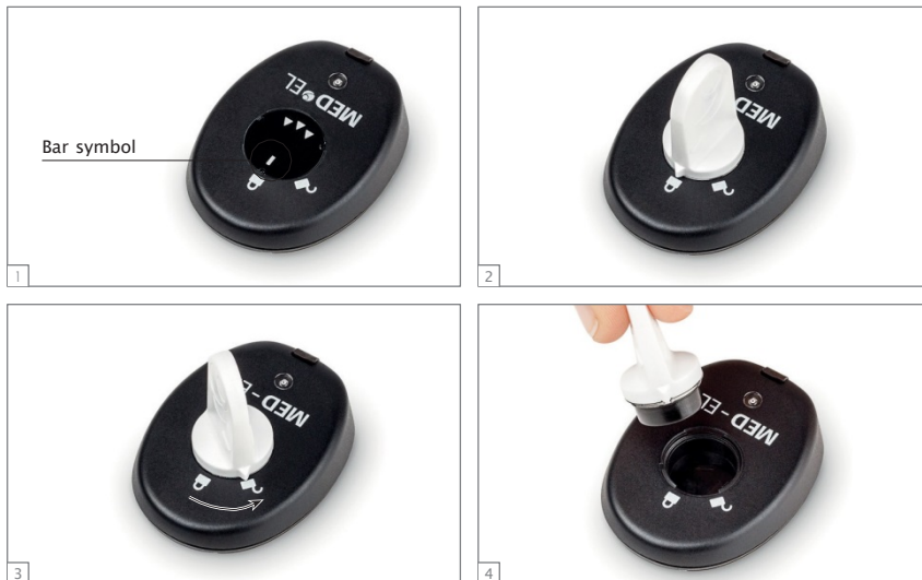
Fig. 11 Changing the magnet
