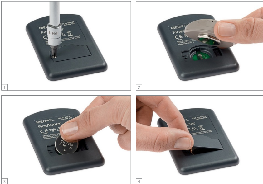
Fig. 18 Changing the battery of your FineTuner
