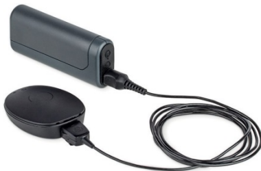
Fig. 14 Mini Battery Pack connected to audio processor
