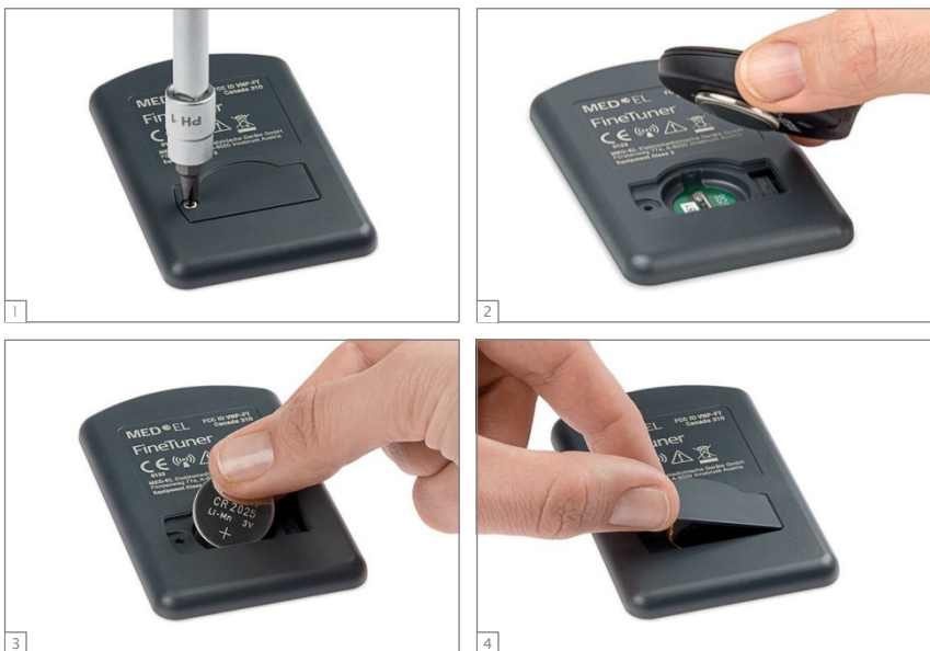
Fig. 16 Changing the battery of your FineTuner
