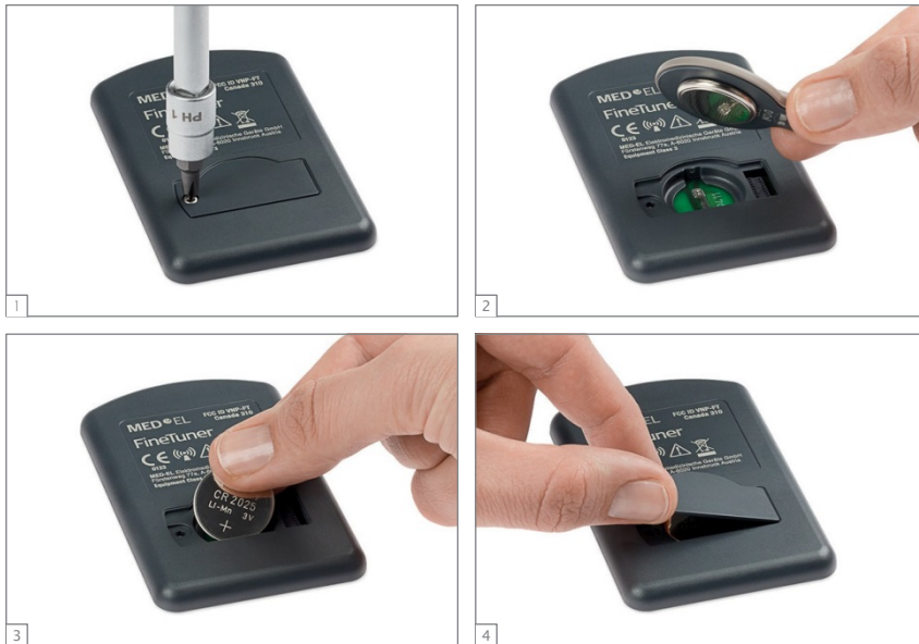
Fig. 36 Changing the battery of your FineTuner
