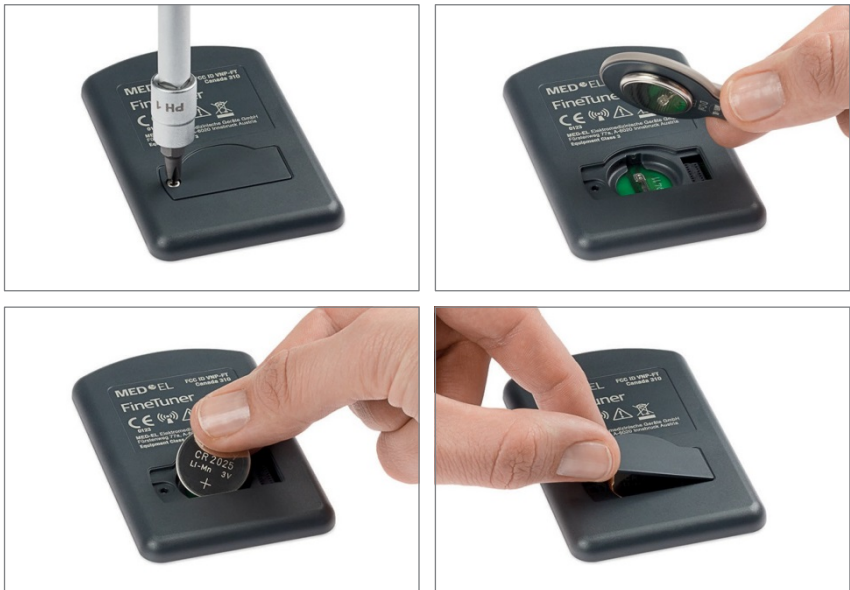
Fig. 25 Changing the battery of your FineTuner
