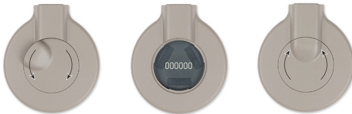
Fig. 9 Removing/inserting the magnet
