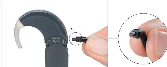
Fig. 28 Plugging the coil cable into control unit
