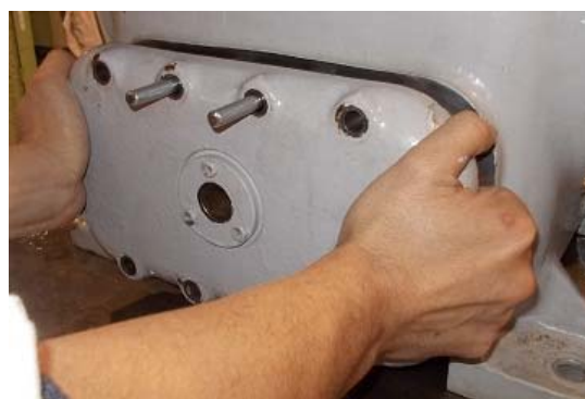
Removal of the Hand hole cover
