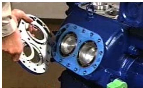
Removing the valve plate
