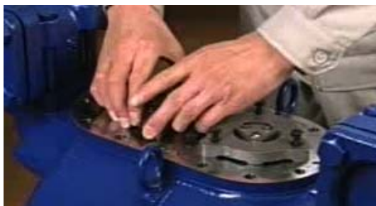
Removal the discharge valve cage
