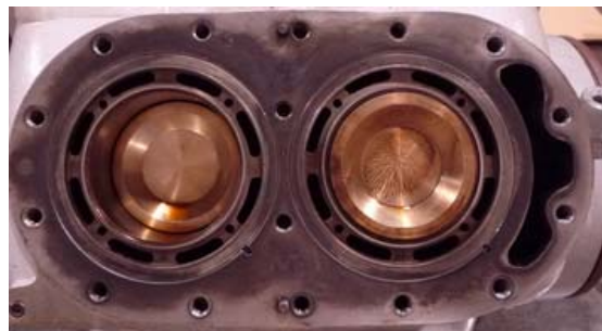
After removing the valve plate
