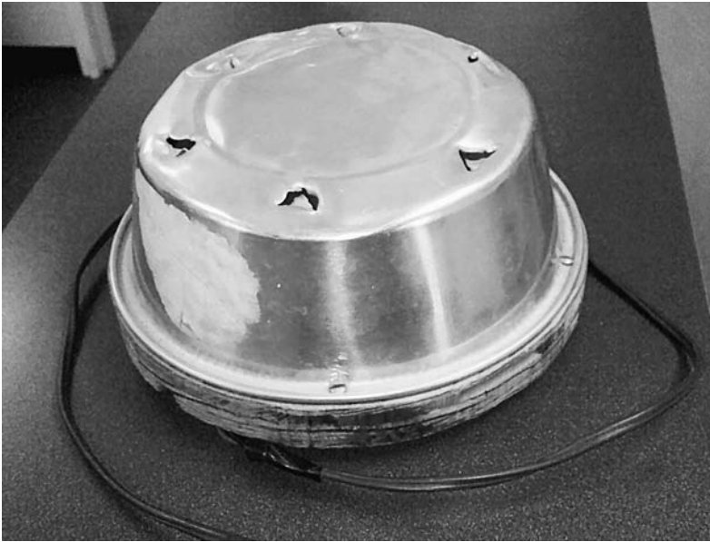
Figure 2.1 The original sound conditioner, housed in a tin saucepan. Photo by author.
