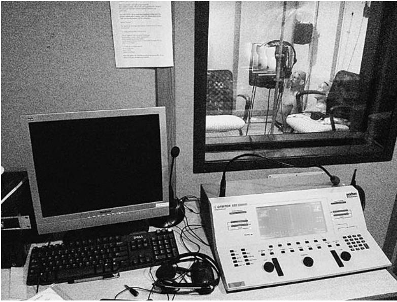
Figure 1.2 An audiometer and, beyond the glass, an audiometric testing booth, part of the research facilities of a hearing aid manufacturer. Photo by author.
