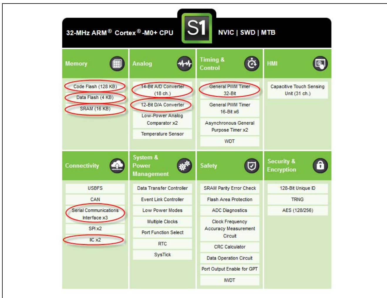
Figure 2. S1 Peripherals used by the simple record example
