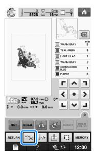
Press **to turn off the automatic thread** cutting function.
