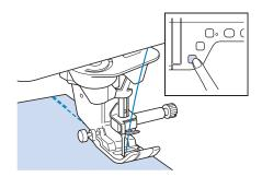
Press the "Thread Cutter" button to trim the upper and lower threads.
