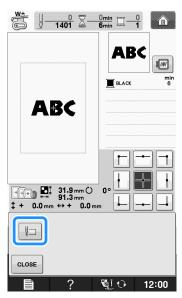
ightarrow The needle is positioned in the lower-left corner of the pattern. The embroidery frame moves so that the needle is positioned correctly.
