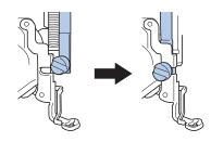
Hold the embroidery foot in place with your right hand, and then use the included screwdriver to securely tighten the presser foot holder screw.
