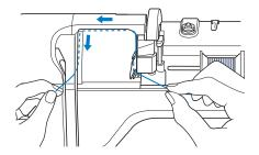
**B** Guide the thread down, up, then down through the groove, as shown in the illustration.
