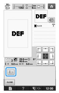
→ The needle is positioned in the lower-left corner of the pattern. The embroidery frame moves so that the needle is positioned correctly.
