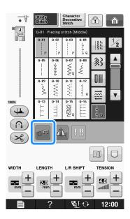
→ The key appears as , the quilting foot is raised to the necessary height, and then the feed dogs are lowered for free motion sewing.
