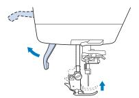
Press the black button on the presser foot holder and remove the presser foot.
