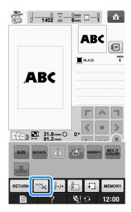
6 Press to turn off the thread cutting function and then press CLOSE.
