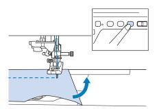
The pivot setting is useful when changing the sewing direction. When the machine is stopped at the corner of the fabric, the machine stops with the needle in the fabric and the presser foot is automatically raised so the fabric can easily be rotated ("Pivoting" on page S-15).
