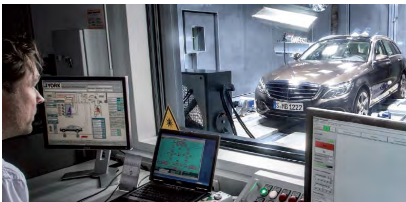
Figure 3-1: Test chamber to measure car cabin emissions
