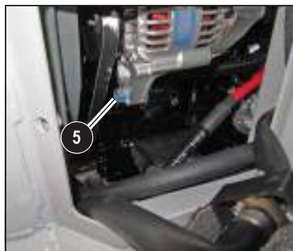
Fig. 33: Slackening the fastening screws
