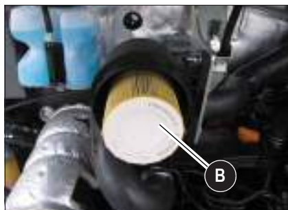
Fig. 24: Removing the outside air filter element
