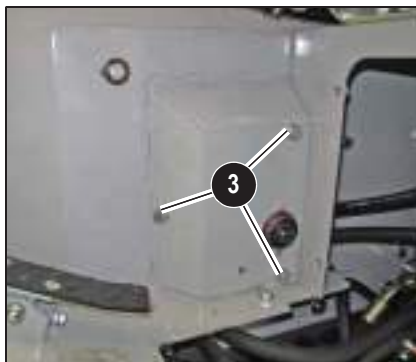
Fig. 31: Slackening the fastening screws
