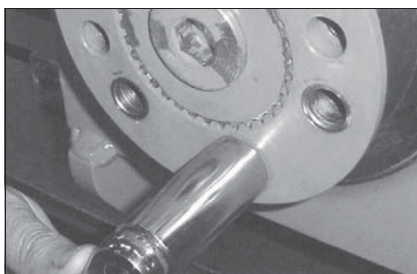
Fig. 65: Removing the bolts
