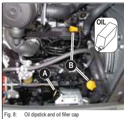
Fig. 8: Oil dipstick and oil filler cap
