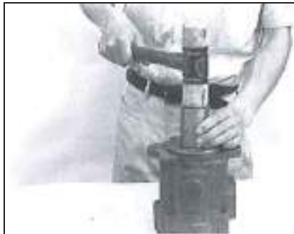
Fig. 15: Fitting the rotary shaft lip seal
