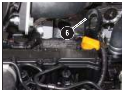
Fig. 34: Removing the shackle
