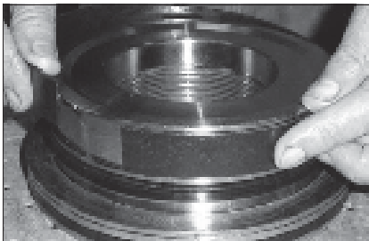
Fig. 36: Coat the seals and surfaces with oil
