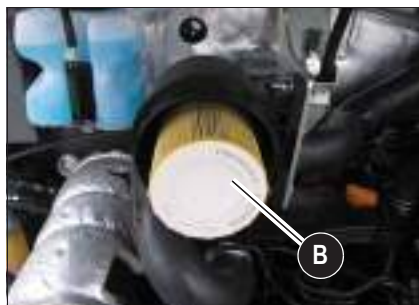
Fig. 24: Removing the outside air filter element
