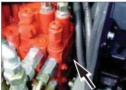
Fig. 6: Main valve block type label
