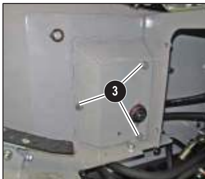
Fig. 31: Slackening the fastening screws
