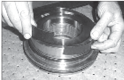
Fig. 24: Removing the seals and bearings
