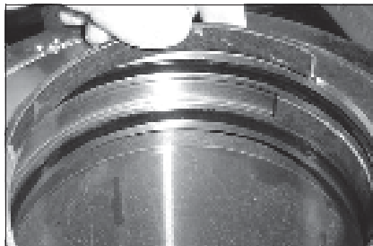
Fig. 40: Fitting the wear indicators
