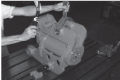
Fig. 10: Removing the standard journal coupling
