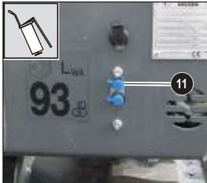
Fig. 79: Lubrication point on ball bearing race of live ring
