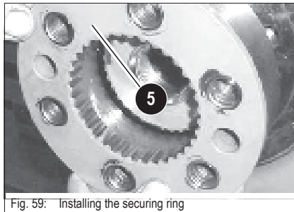
Fig. 59: Installing the securing ring
