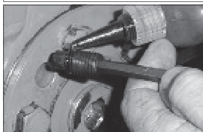
Fig. 73: Loctite 545 on set screws
