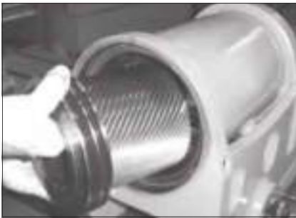
Fig. 21: Removing the piston tube with a hammer and drift
