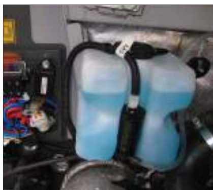
Fig. 6: Tank for washer system
