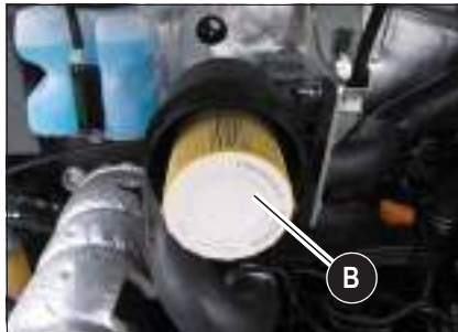
Fig. 21: Removing the outside air filter element
