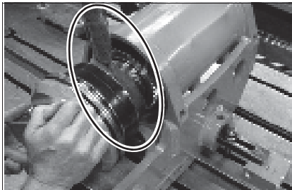
Fig. 52: Inserting the shaft
