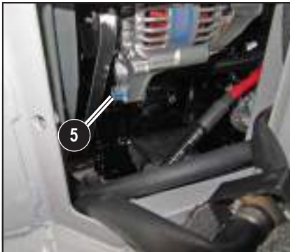
Fig. 33: Slackening the fastening screws
