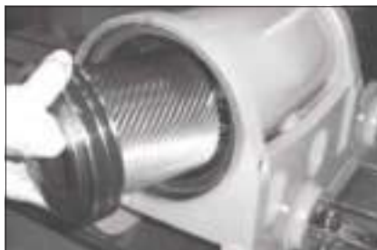
Fig. 48: Fitting the piston tube
