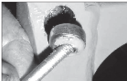
Fig. 27: Removing the grease nipple, etc.
